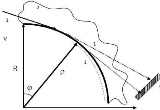
Fig. 8.1. A scheme of the neutron centrifugal experiment. 1: classical trajectories of incoming and outgoing neutrons, 2: cylindrical mirror, 3: neutron detector, 4: quantum motion along the mirror surface.
